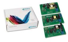
Dialog has evaluation boards for 10W and 15W single-output power supplies, as well as 15W dual-output supplies. These evaluation boards use standard, easy-to-procure components, including transformers from Wurth Electronics Midcom, and enable customers to evaluate Dialog's <a href="https://www.iwv1830">iW1830</a> AC/DC converters, with their high efficiency, low no-load power consumption, excellent EMI performance. Download evaluation board documentation on the
