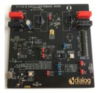
Groundbreaking! that's the DA9313 high-voltage power management integrated circuit (PMIC) with a maximum output current of 10 A, suitable for applications supplied from a dual (2S) Li-ion or Li-polymer stacked cell battery pack, or any input voltage between 5 V and 10.5 V. The IC operates with efficiency during conversion of up to 98 %. Master/slave operation is offered, where a pair of devices can combine to double the peak output current to 20 A.
